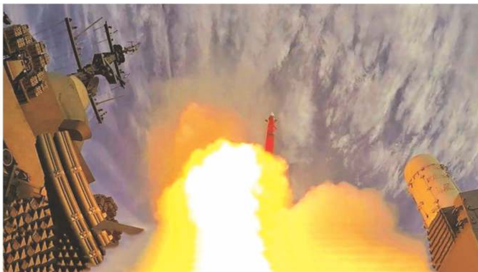
Two LRSAM launchers that can send eight 150-km-range radio frequency SAMs.
