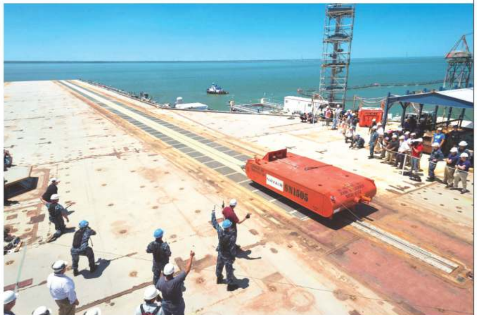
EMALS catapults being demonstrated on the aircraft carrier Gerald R. Ford (CVN 78), with weighted sleds off the ship into the James River, 16 June 2015.
