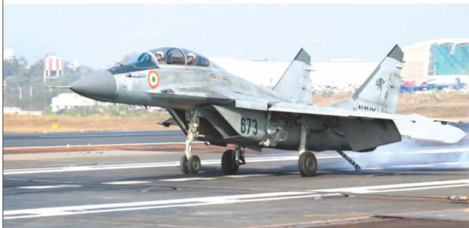
An Indian Navy MiG-29K jet seconds before engaging an arrestor wire on landing at a Shore Based Test Facility in Goa.
